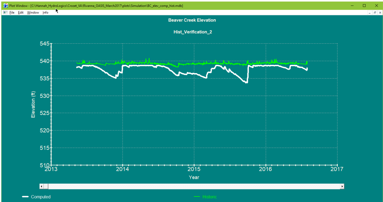
Figure 8: Original Model Verification Using Spillway Outflow Meter
