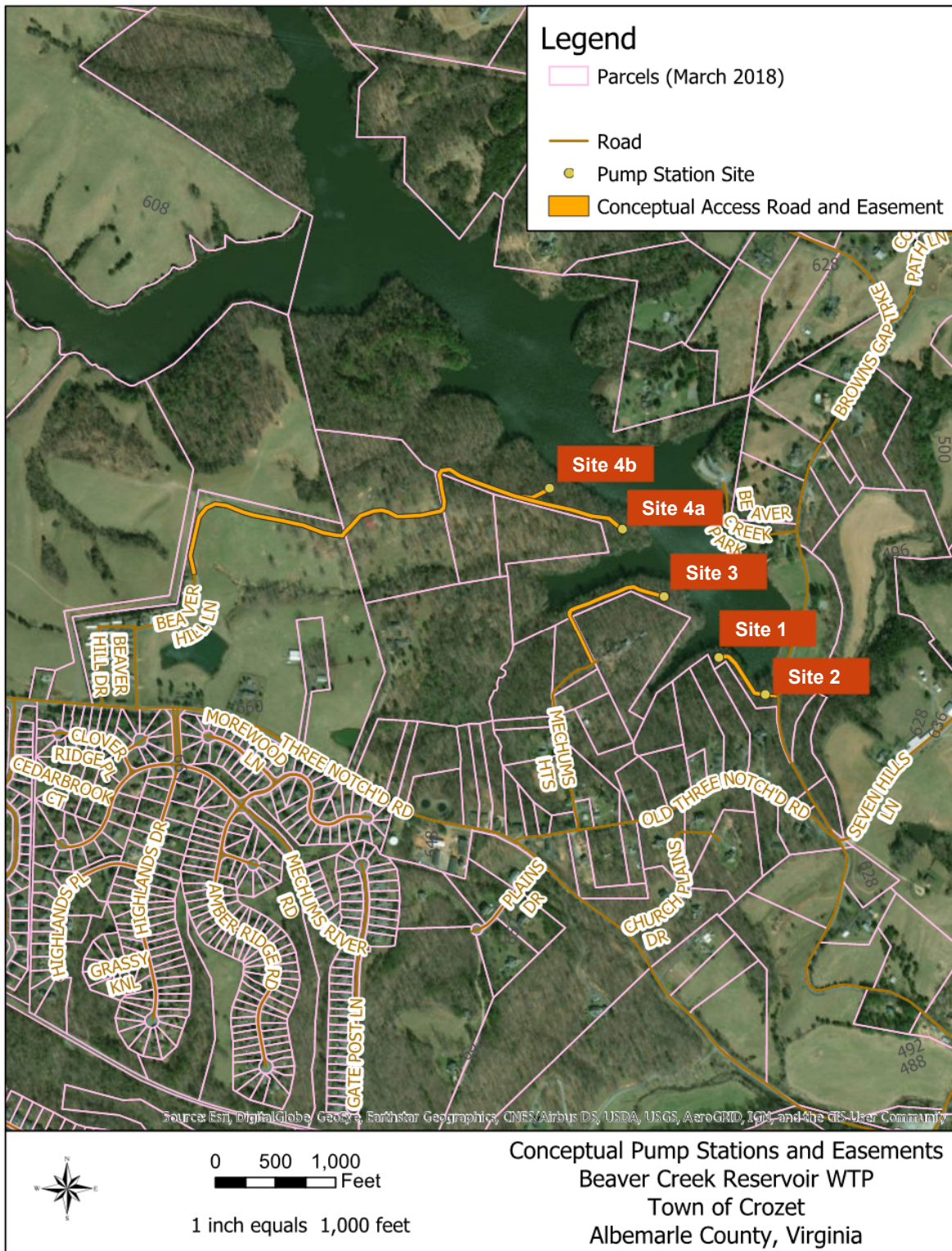
Figure 4-8: Pump Station Sites with Conceptual Roadway/Waterline Easements
