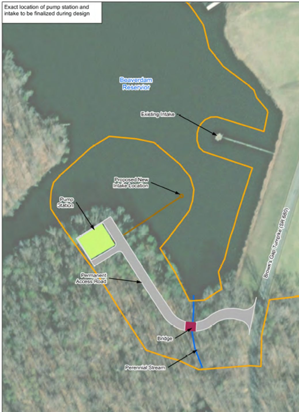
Figure 9.1 – Maximum Limits of Disturbance – Pump Station
